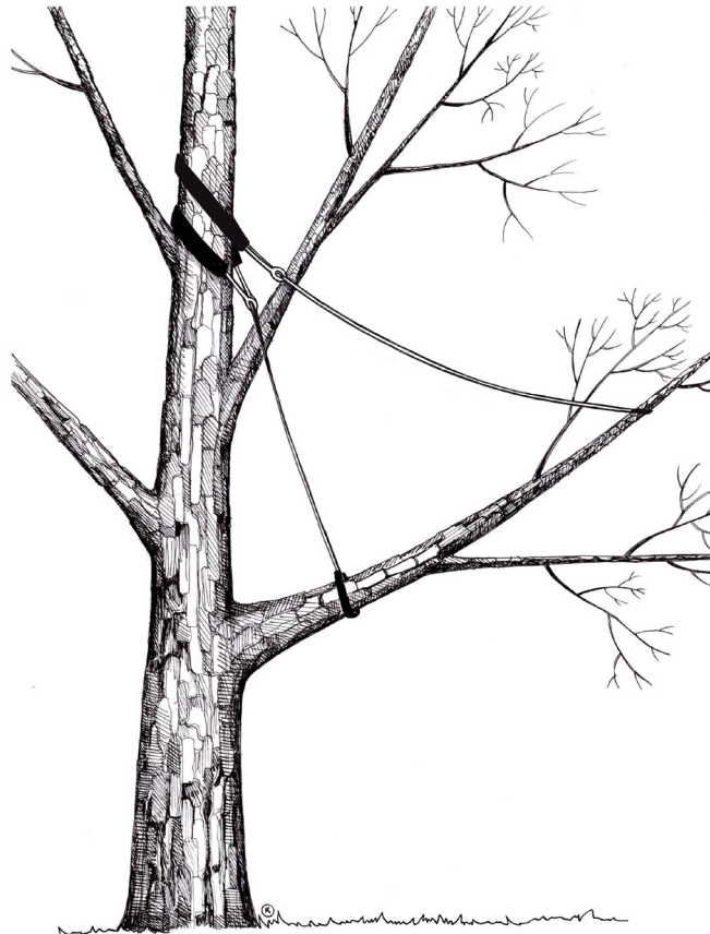
Figure 6: Securing a horizontal branch to prevent damage in the event of failure
